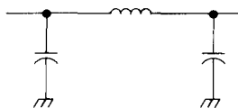
fig. 1. The pi network is so named because of its basic resemblance to the Greek letter \pi .
